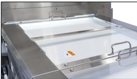
Stainless steel body and a 650mm wide belt with lightweight protective cover.
